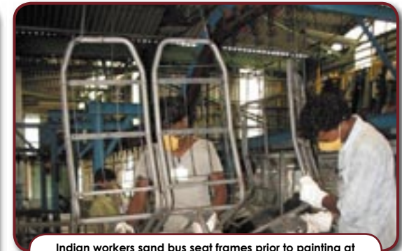
Indian workers sand bus seat frames prior to painting at Pinnacle Industries. These workers can easily transfer their skills to the manufacture of wheelchairs.
