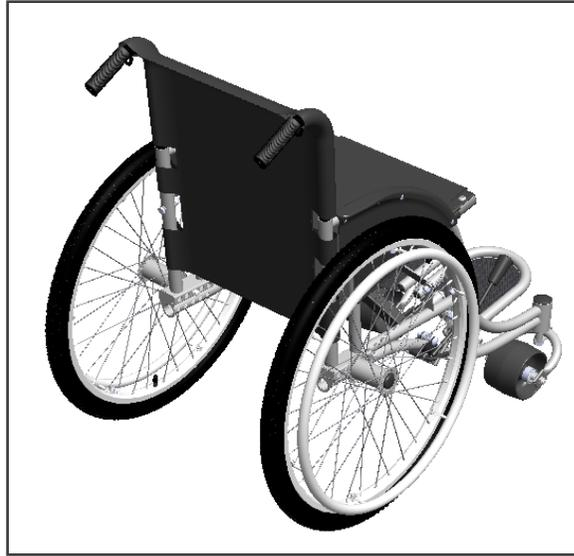
**1.** While depressing the large black button: put the axle completely through the hub and then place one large spacer on the axle so that the spacer goes between the wheel and the frame.
