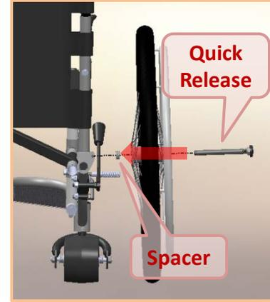
**3.** Make sure the quick release detente (ball) passes completely through the axle block so that the axle will not slide out unintentionally. Release the black button and the axle will be locked in place.
