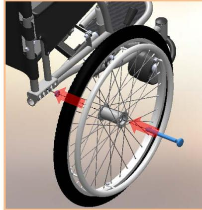
**2.** Put the axle through the desired axle hole, making sure that left and right wheels are mounted in the same position.
